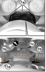
Remove the upper part (1a) of the steering column, releasing its inner side retainers (1b).
